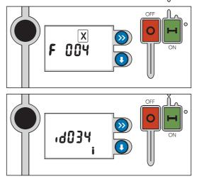
RC-id settings of the power supply and Remote control unit. New match between the power Supply and the RC has to be made according to the instruction in the RC unit only when this message is displayed
